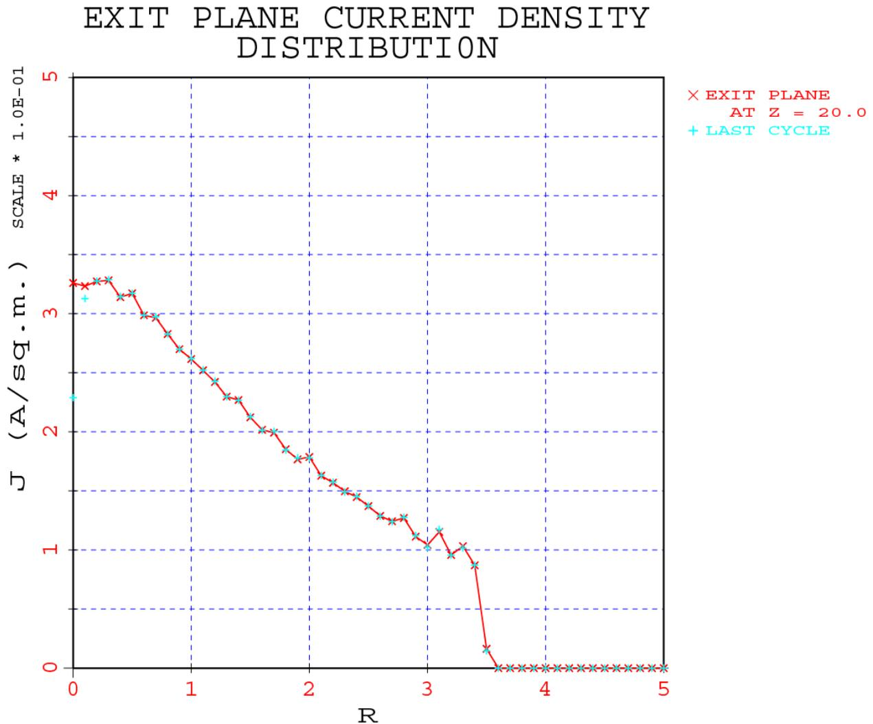
Figure 63: Current density distribution at exit plane of CRT gun
