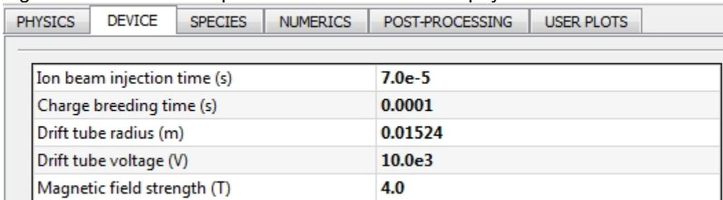
Figure 6: DEVICE tab: the parameters that are related to the EBIS device and operation.
