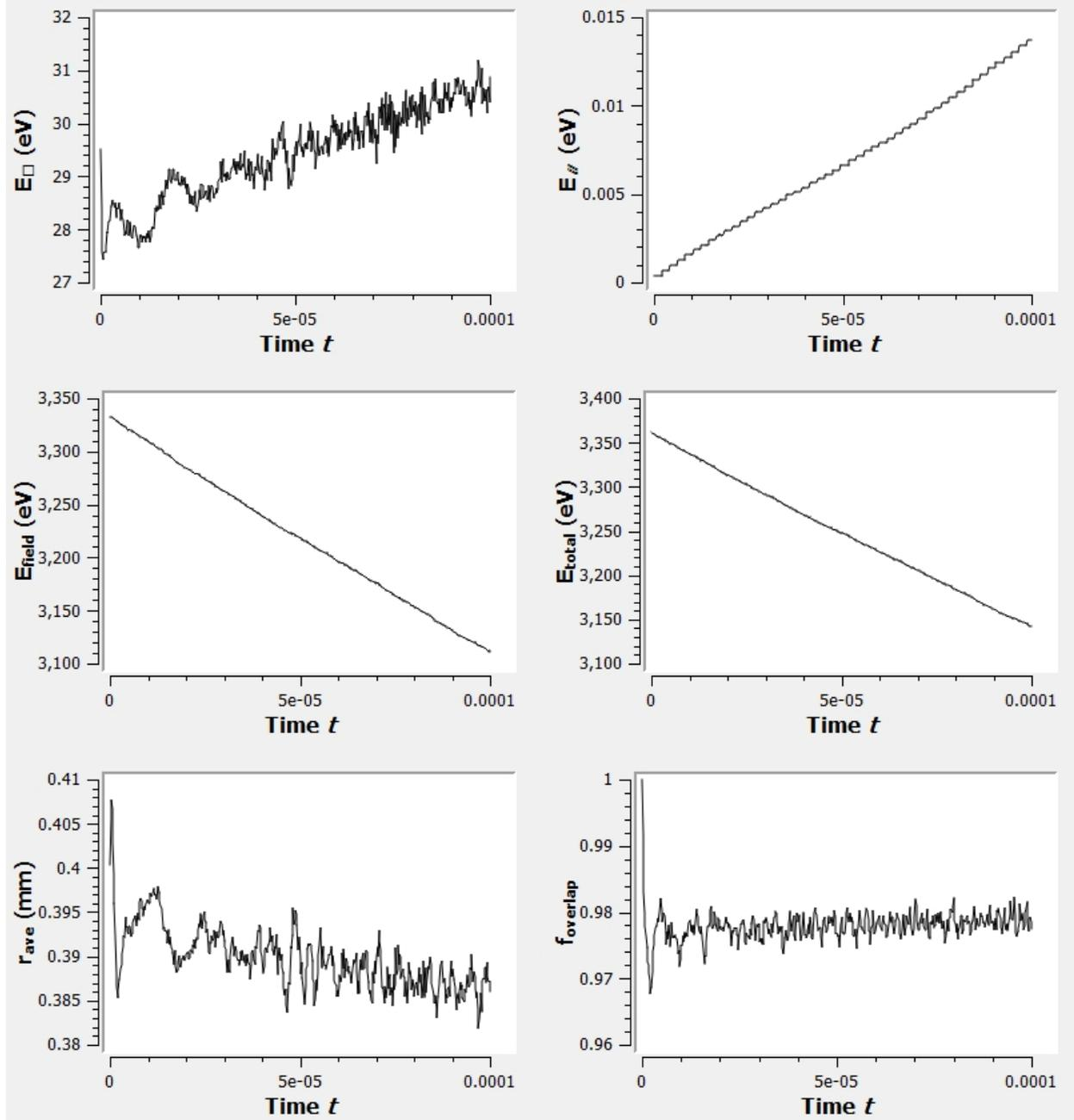
**Averages:** Time evolution of averaged 1) perpendicular energy; 2) parallel (axial) energy; 3) field energy; 4) total energy; 5) average ion radial position; 6) ion overlapping percentage with electron beam.
