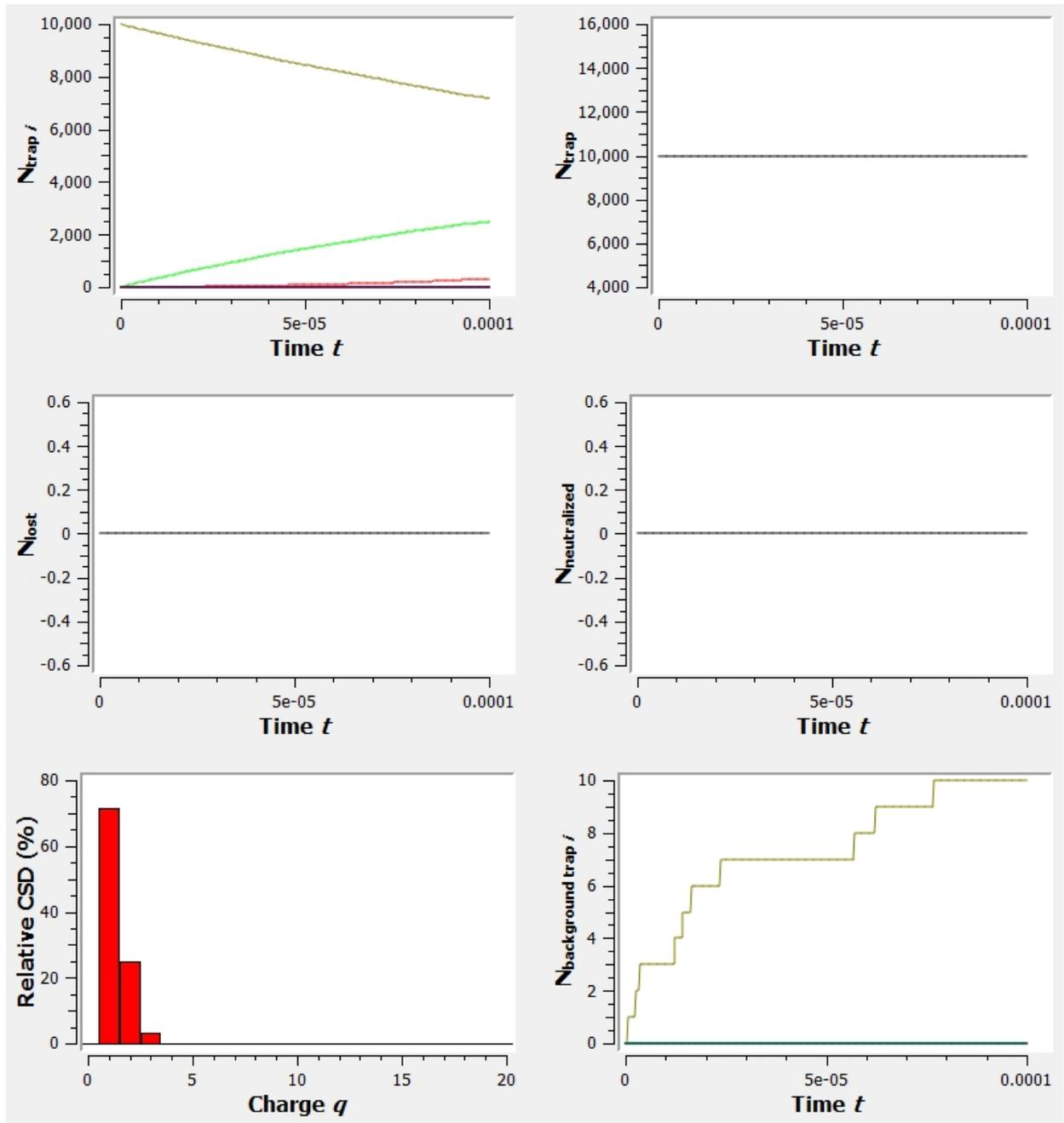
**Counts tab:** time evolution of 1) ion charge states; 2) number of trapped particles; 3) number of ions that are lost to the wall; 4) number of neutralized ions; 5) relative charge state distribution; 6) number of the neutral gas ions.
