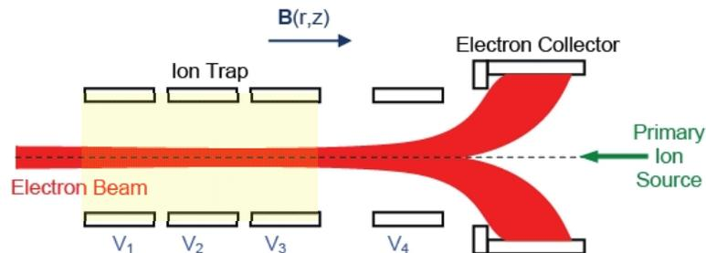
Figure 1: Diagram of EBIS device. The electron beam travels to the right until stopped by the electron collector. The primary ion source is to the right of the collector. The ion trap is indicated by the shaded region.
