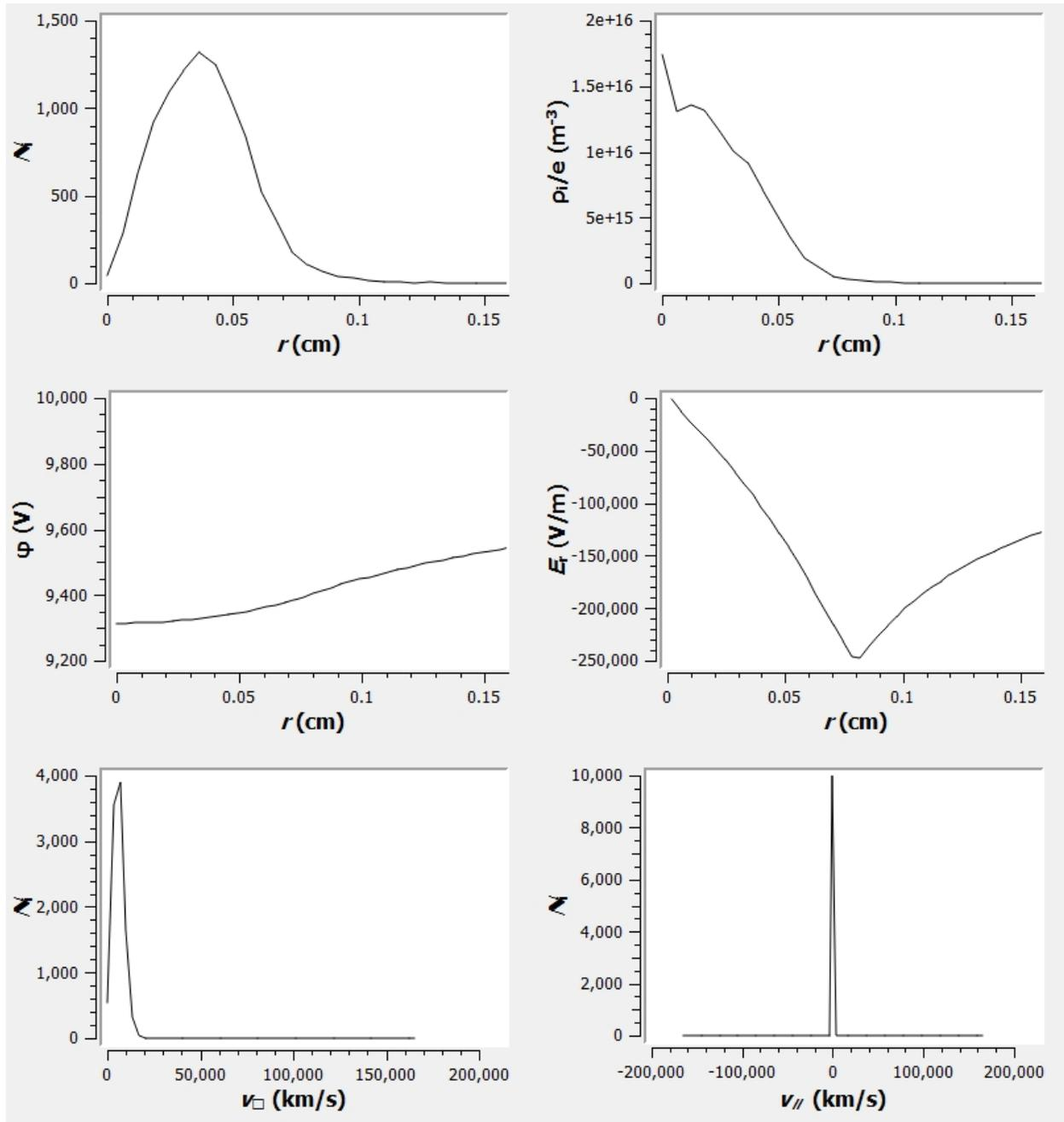
**Profiles tab:** Radial distributions of 1) ion number; 2) ion charge density; 3) potential; 4) electrical field; 5) perpendicular velocity distribution; 6) axial velocity distribution.
