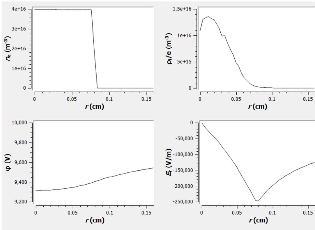
**Final Plots tab:** Radial profiles of 1) electron density; 2) ion charge density; 3) potential; 4) electrical field.
